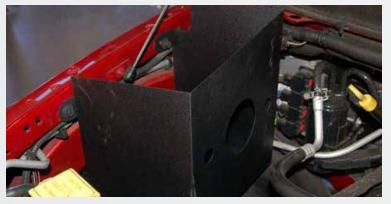
Install the BBK air filter shield inplace on inner fender. Secure with the stock (2) bolts.
