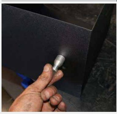
Install the supplied aluminum pins to the bottom of the air shield using the supplied screws.
