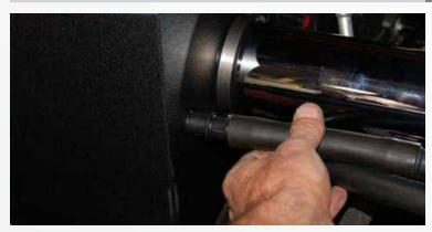
Insert the supplied 5/8" black plastic hose connector into the hole in the base of the filter, connect the stock breather hose to the black connector. If you need a little extra length In the breather hose, loosen the clamp at the other end of the hose, where it connects to the engine and turn the hose toward the air filter.
