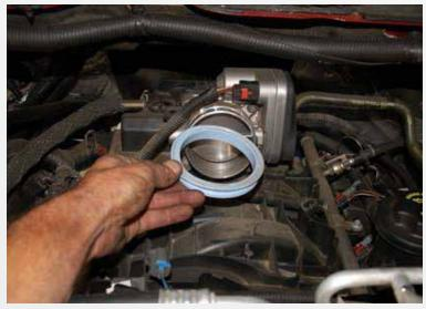
Loosen the two bolts that hold the plenum to the intake manifold. Remove plenum. Remove rubber seal from throttle body.
