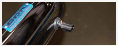
Install the supplied black rubber grommet in the chrome inlet tube. Install the Intake Air Temp (IAT) sensor that you removed from the stock plenum in STEP 2, into the grommet.
