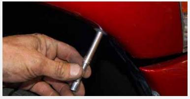
Remove the seven (7) inner fender screws from under the fender.
