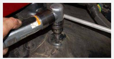
Earlier model pickups have rubber grommets on the bottom of the stock air box. Remove And install on these aluminum pins. Later model pickups have screws that held the air box Mounting bracket to the inner fender. If yours has the screws, then drill out the screw holes In the plastic inner fender to 9/16". Then the aluminum pins will locate in the holes.
