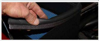
Install sponge seal to top of air filter shield. Trim off extra.
