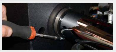
Take the clamp off the neck of the supplied air filter and place on chrome inlet tube, on the engine side of the shield. Install the filter onto the tube and line up the breather hole in the filter base with the forward hole in the shield. Place clamp on neck of filter and tighten.
