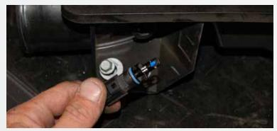
Unplug Intake Air Temp Sensor. Its located in the front of the decorative plenum box, just to the right of the inlet hose connection. Turn sensor to the left to unlock and remove.
